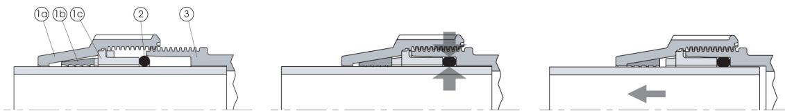
Sealing mechanism of the fitting range 75 to 110mm
